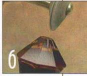
(Photo 4) Set angles to cut 8 main facets followed by 8 small star facets. Polish all facets in a way appropriate for gem material you are using.
